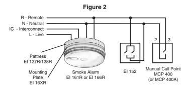
7.Connect the mains power – the green LED light on the alarm should be on. When the test button is pressed the horn should sound.
